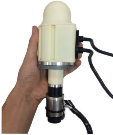
Figure 5. CAD modelling and developed prototype of the tendon driving unit for the assistive glove. The underlying working principle is the same one of the elbow unit, outlined in Figure 3(a). The unit is actuated by a brushless DC motor (b) with a reduction gearhead of 23:1 (c) whose angular position is monitored by a rotary encoder (a). An electromechanical clutch (f) allows to lock the system and keep the hand in place in a low-power state. An array of 6 spools (d), dimensioned according to the first hand postural synergy pulls and release a set of tendons routed through the glove. A pair of spur gears (e) transmits power from the motor to the spool with a reduction of 3:1. A feeder mechanism (g) keeps the tendons in tension around the spools.
