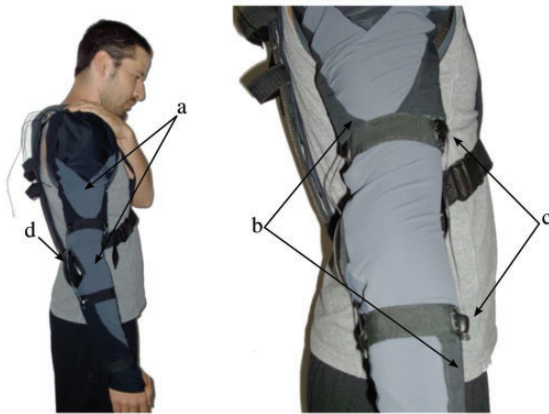
Figure 10. First prototype of the elbow sleeve. (a) Stretchable fabric. (b) Load paths made of nylon webbing for efficient transmission of the forces applied by the tendons. (c) 3D-printed anchor points. (d) Semi-rigid elbow protection. The sleeve, including bowden cables, weighs less than 200 g.
