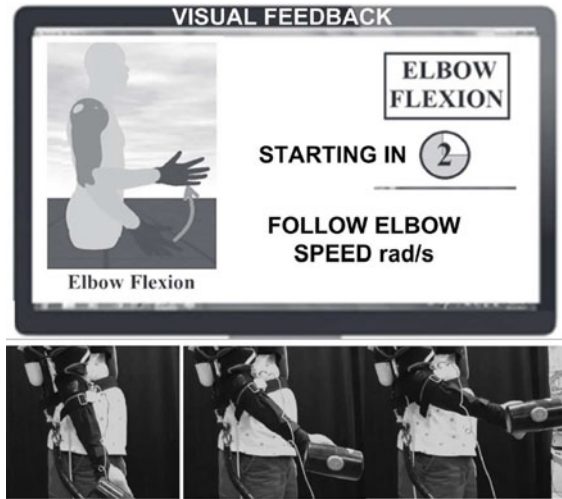
Fig. 4. The experiment was run by instructing the subjects to replicate the movements of a virtual avatar on the screen, trying to match the elbow speed.
