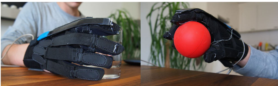
Figure 1. The soft, synergy-based robotic glove for grasping assistance.
